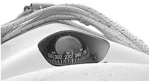
Sea kayak compass: mounted ahead of forward hatch so that horizon is in paddler's peripheral vision
