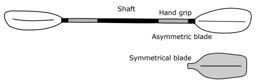
Blade shapes may vary, but the asymmetric shape, which reduces twisting, is now common in kayak paddles. Blade sizes also vary, and the temptation may be to use large blades thinking that they will give more power. However, bigger blades, especially on longer shafts, can lead to joint injuries. It's best to take advice before spending too much.
