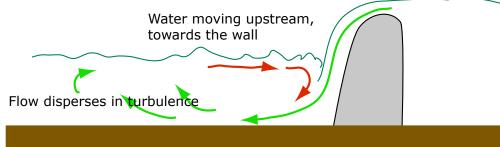
The problem with weirs is that water circulates on the downstream side, and there is no escape to either side, as there is with isolated rocks. Any floating object in that circulating flow can be trapped indefinitely. Portage.
